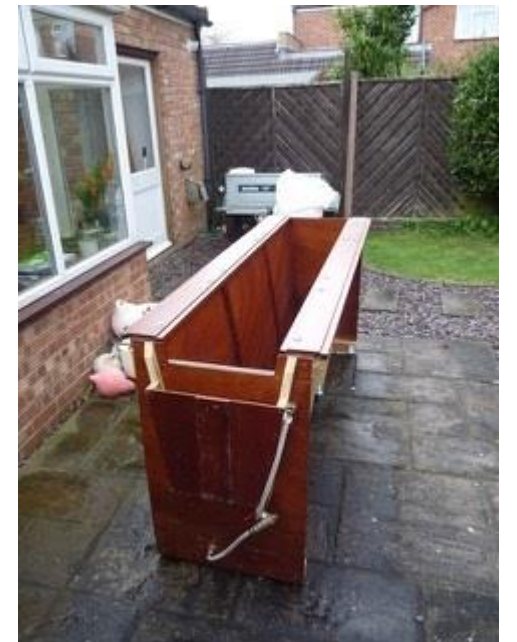
6. Assembled tank showing weir end drainage pipes
